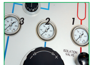
The three pressure gauges indicate: 1. pressure in bottle 2. pressure set by pressure regulator 3. pressure at test port
