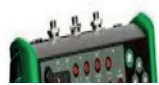
The internal pressure modules connections are located on the top of the MC6 calibrator. There is enough space to easily connect the test hose to the module.
