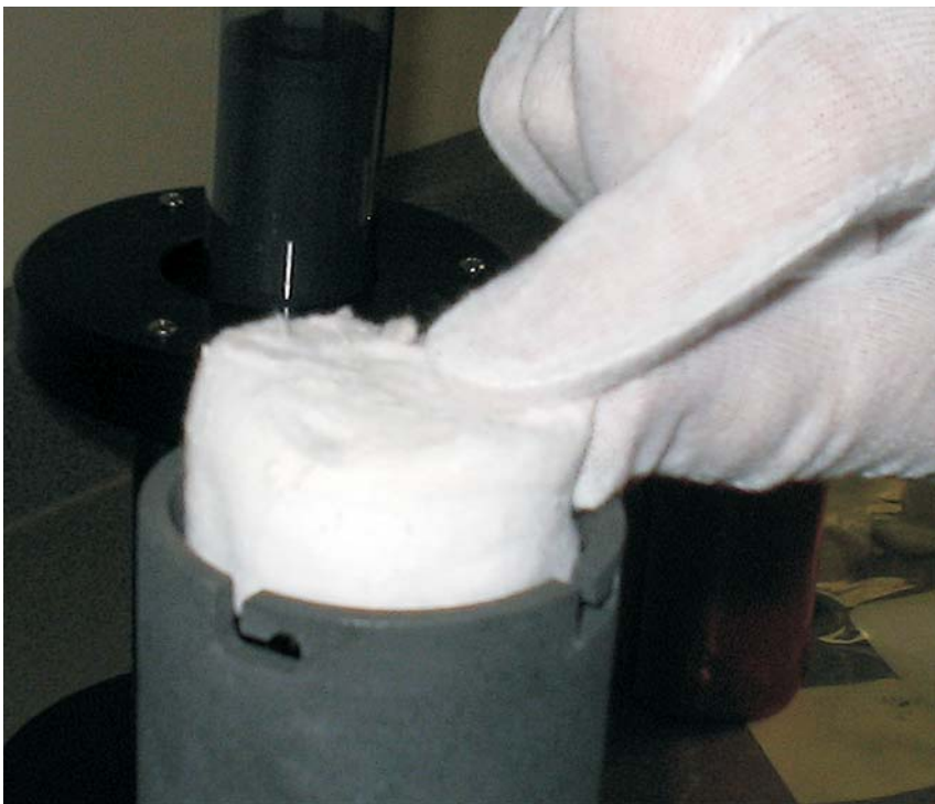
Figure 16 Place insulation in cell basket
