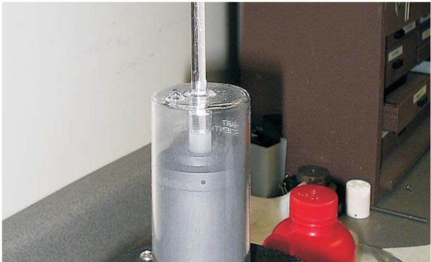
Figure 14 Push insulation to bottom of re-entrant well.
