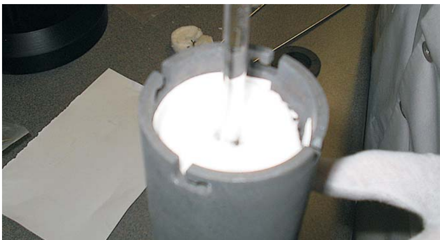
Figure 22 Fiber ceramic insulation installed on top of cell.
