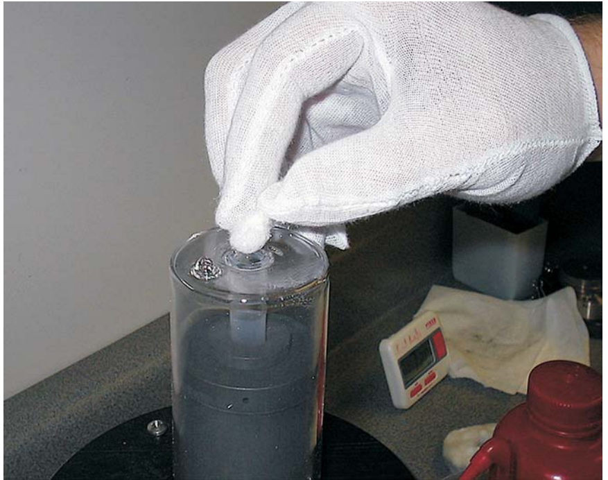
Figure 13 Place insulation in re-entrant well.
