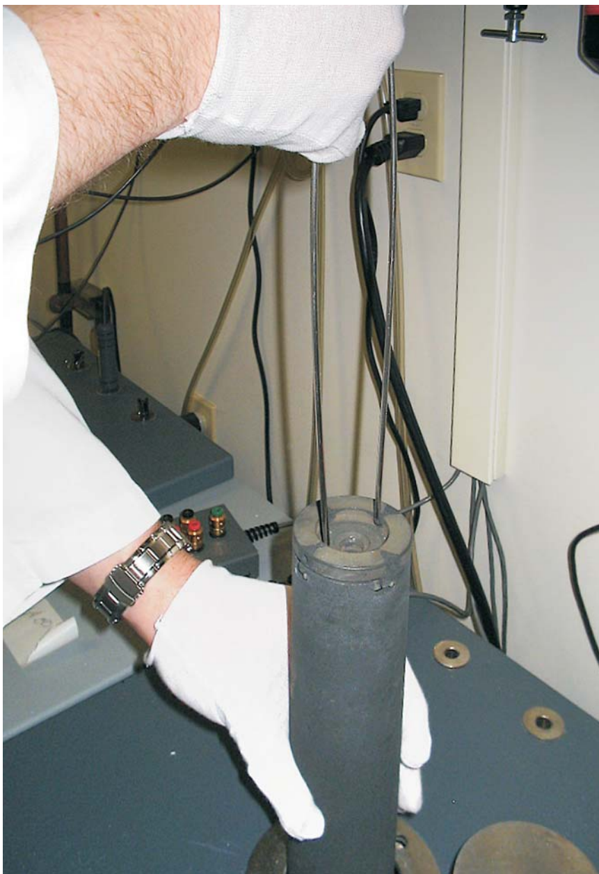
Figure 25 Installing basket assembly in furnace.
