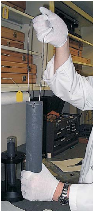
Figure 24 Preparing basket assembly for installation in furnace.
