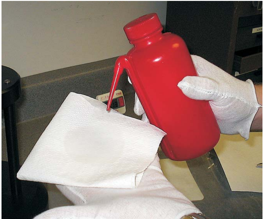
Figure 11 Preparing paper towel with reagent grade alcohol.
