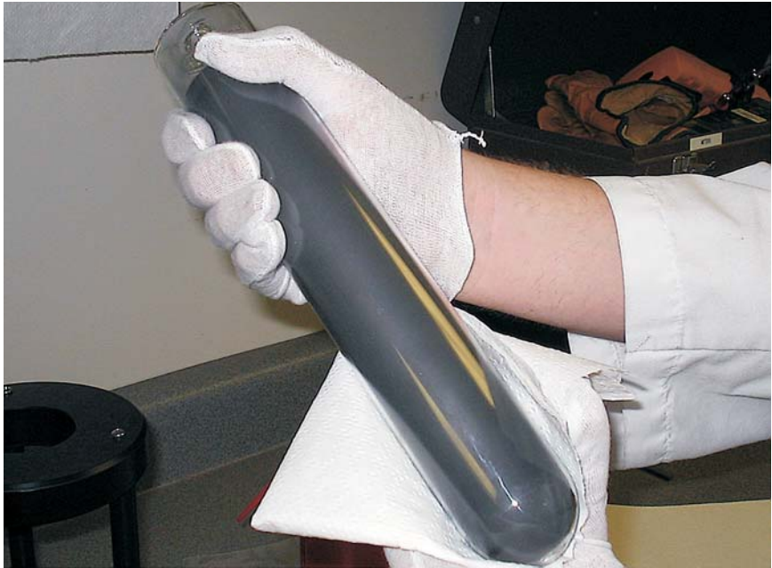
Figure 12 Clean cell completely.
