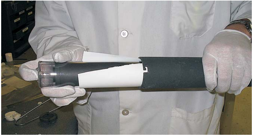
Figure 20 Insert cell into basket.
